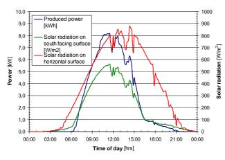
**Figure 3**. PV generation versus solar radiation for June 23 – 2001. The curves show measured data for the PV wall. On June 23. the solar radiation on the vertical south facing facade was 550 Watt/m2 at 12:00 am. For the 100 m2 PV wall the solar radiation was 55 000 Watt (55 kW). The measured power was 8 kW, which indicates that around 15 % of the solar radiation was transformed into electricity.
